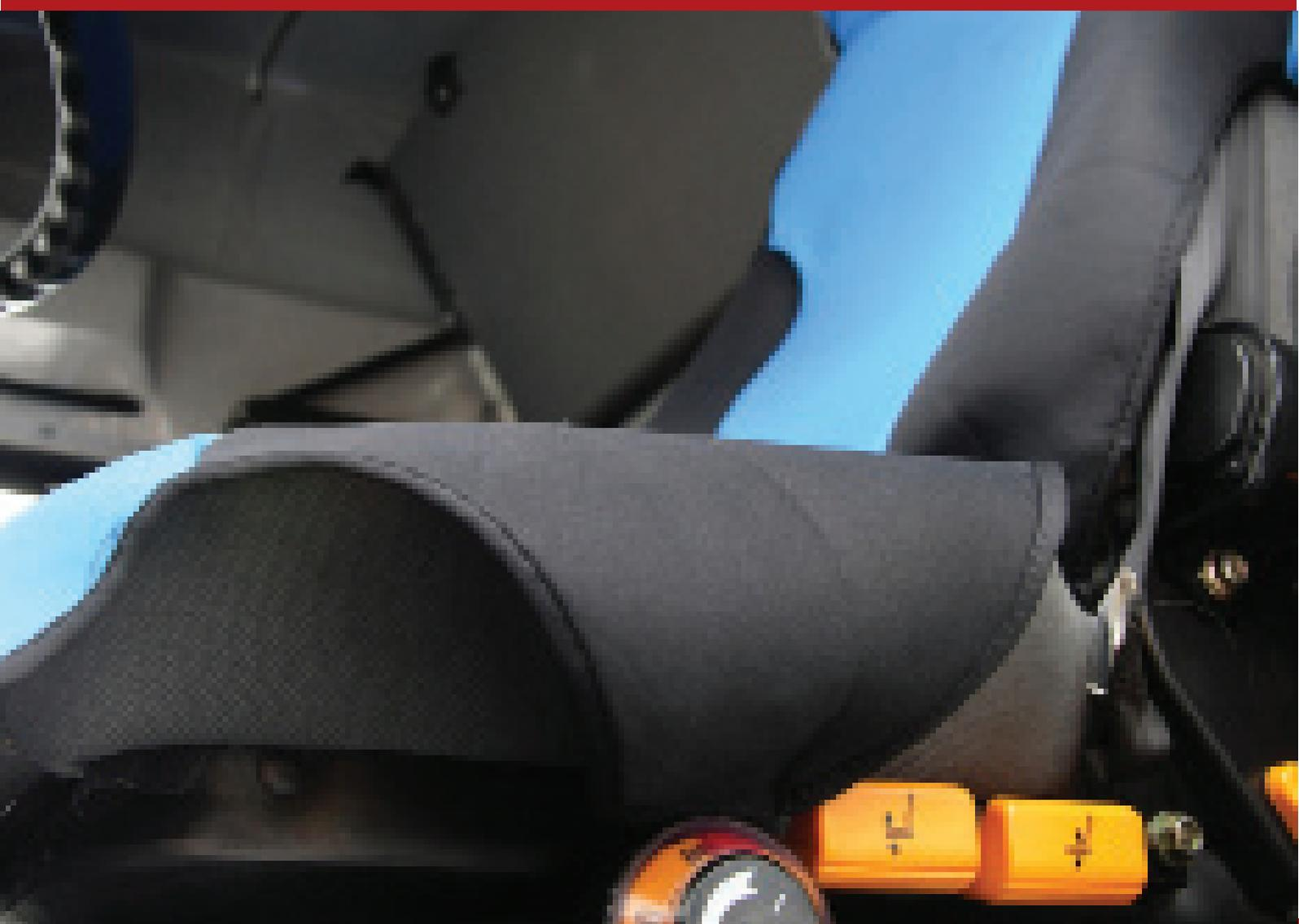
A Prosig P8000 system is used to measure vibrations at defined points on seats designed for commercial / industrial / agricultural vehicles. The seats are tested on a 3-axis shaker rig while suitably loaded. The DATS Human Response software is then used to check that the seat complies with the relevant standard.
