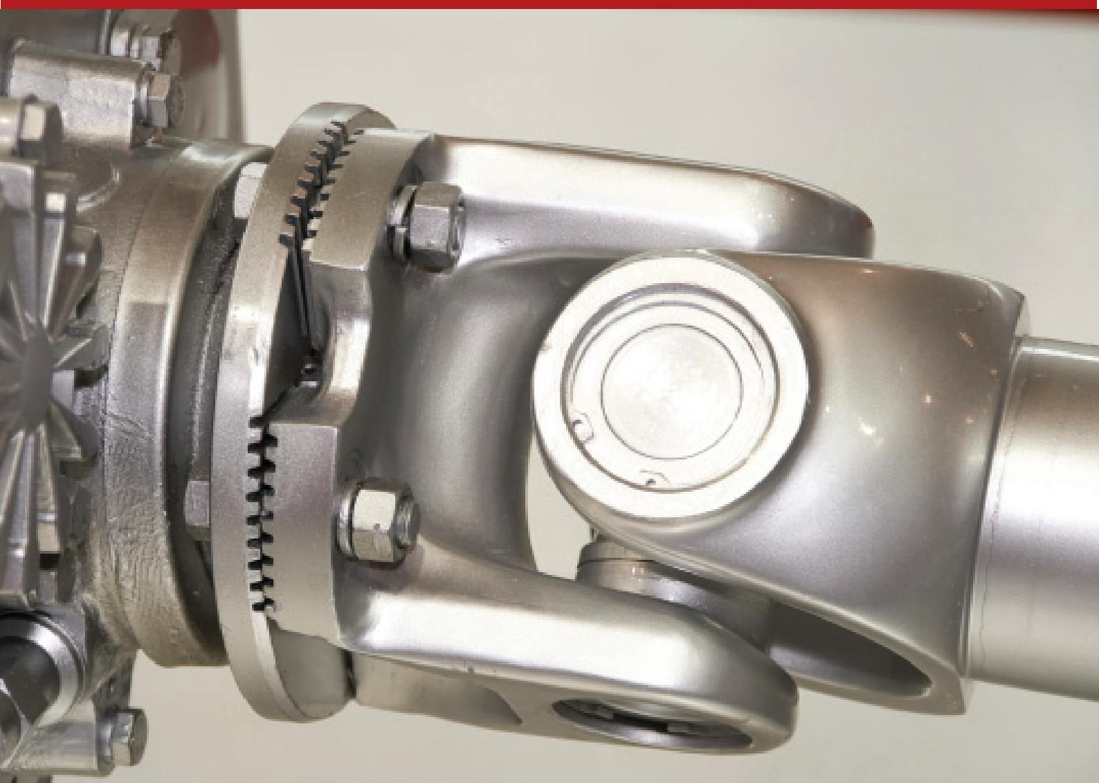
Transmission Error, also called Torsional Vibration, is the study of the rotational speed of a rotating object. A shaft will not normally rotate in a smooth motion, but will actually accelerate and decelerate as it moves around its cycle. This is an important factor in the refinement of any machine or device that has rotating parts.
